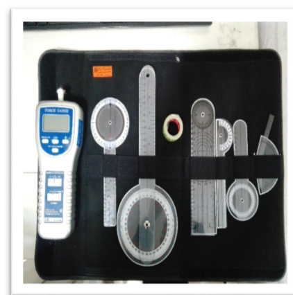
Fig. 2. Measurement set (goniometer and algometer)
