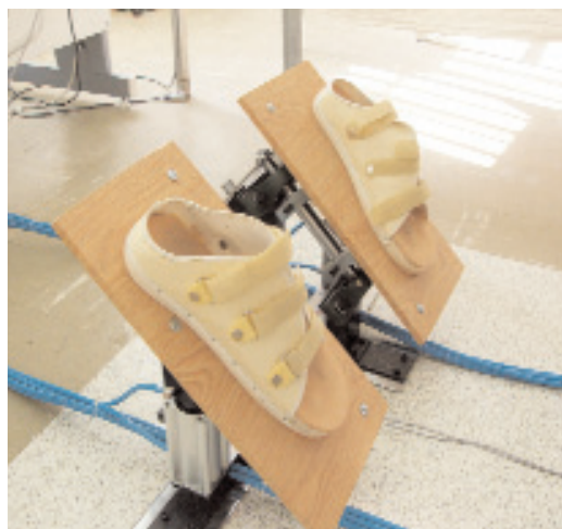
Fig.1a. An Illustration of Oblique Platforms of New Designed Ankle Perturbation System (APS).
