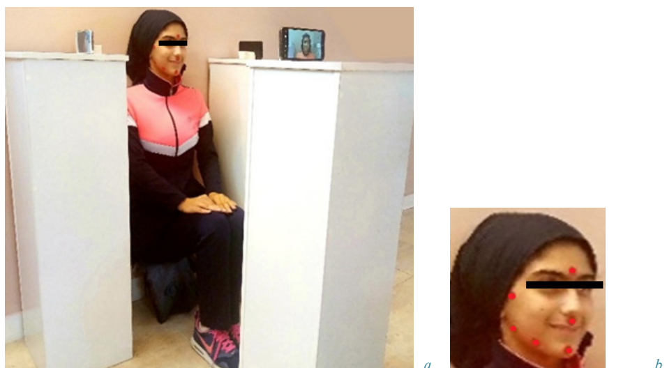
Figure 1. Cameras (a) color markers (b) adjusting and preparing the system for recording facial symmetry and mandibular movements with three mobile cameras.
