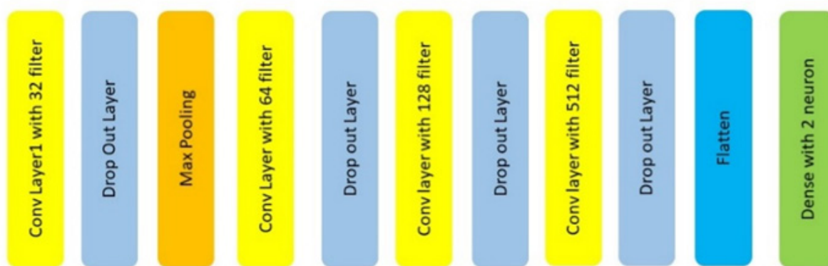
Fig. 3. Base Model Architecture
