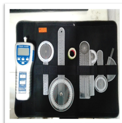
Fig. 2. Measurement set (goniometer and algometer)
