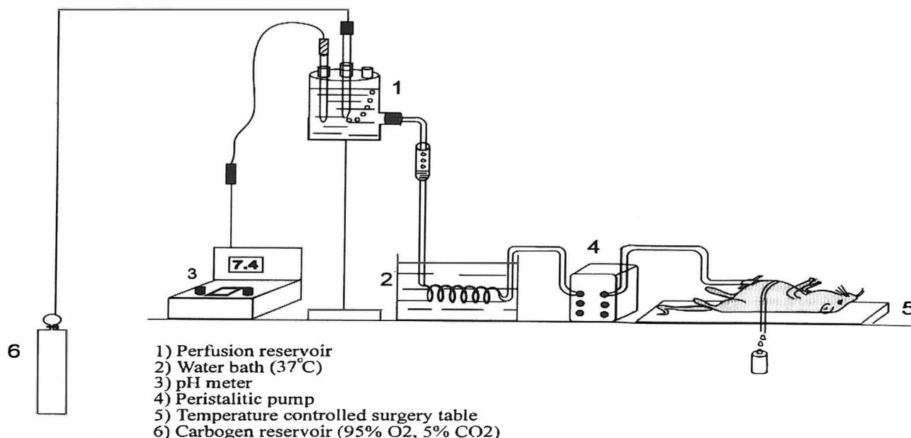
**Fig. 1.** Schematic diagram of a rat liver perfusion system. Catheters are inserted into the portal vein and inferior vena cava. Perfusion is pumped from a central reservoir by an oscillating pump through an 80  $\mu$ m nylon filter. Before entering the liver oxygenation takes place through an oxygenator containing 95% O<sub>2</sub> and 5% CO<sub>2</sub>.
