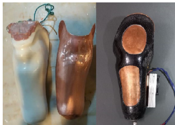
Figure 1. A new socket with a heat-exchanging metal layer and filled mold with silicone top(left); the final socket (Right)
